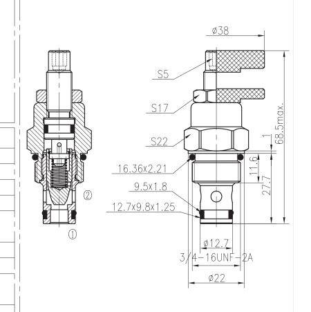
The valve reduce its office value from fully opened to fully close with clock—wise adjustment rotation.
