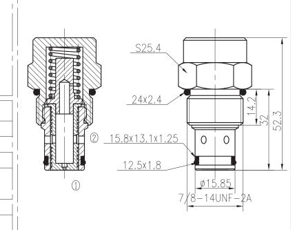
The valve maintains a constant flow rate out of © regardless of load pressure changes in port ©. That is to say, when flow from © to © to through the control office is compensated and reverse flow from © to © returns through the control office and is non—compensated.
