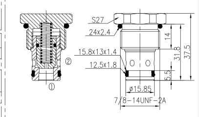
The valve allows flow from ② to ① with very low pressure drop, while blocks flow from ① to ② .
