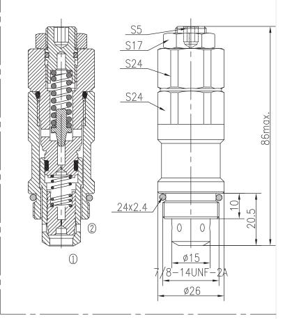
The valve blocks flow from 0 to 0 until 90% pressure is present at O.With the continued increase pressure on 0,0 to 0 began to overflow, until to the spring's maximum pressure.
